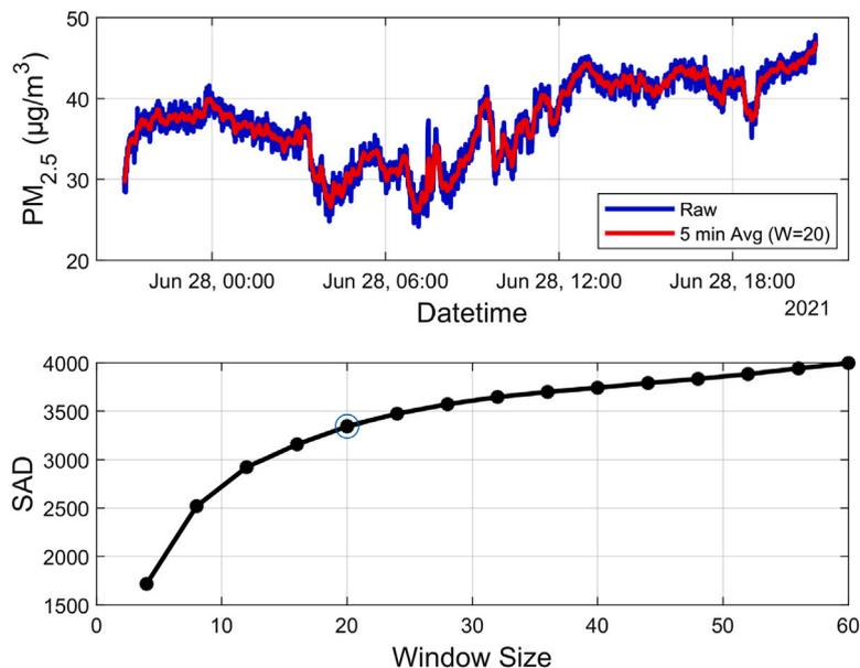
Fig. 1. Using the sum of absolute difference (SAD) to determine window size. Here we can see the SAD starts to plateau around a window size of 20. The raw data is 15 s resolution, so a window size of 20 corresponds to a 5 min moving average.
