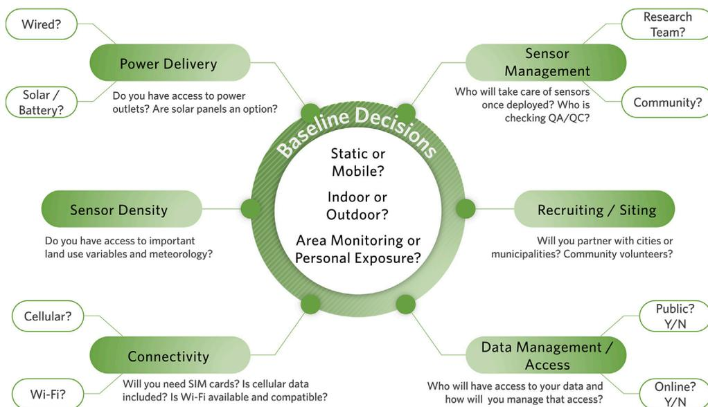
Fig. 2. A summary of key decisions that are required when developing your sensor network.
