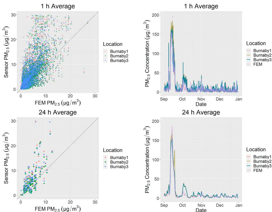
Fig. 3. FEM data compared to three PurpleAir monitors (Burnaby 1–3). Comparisons are shown both as a scatter plot (left) and a time series plot (right).
